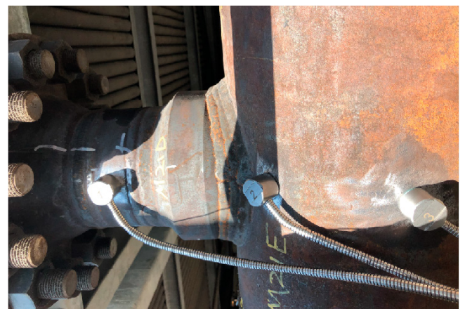
Figure 9: Dual-Element UT sensors with optional SS cable jacket.
